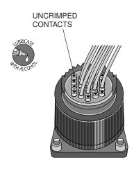
8. Check the mating face of the connector to insure that all the same size contacts are on the same plane (fully inserted). If not, the contact is not fully inserted. Remove the contact using the proper extraction tool and procedure and re-insert. Do not attempt to reinsert the insertion tool to correct the problem.
