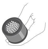
A wire hole filler must be inserted into the grommet behind the unused contacts to maintain the sealing integrity of the connector.
