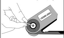
6. Insert the stripped wire into the contact with a slight twisting motion. Be sure all wire strands are inside the contact. Squeeze the handle to cycle the tool. The handle will not release until the contact is completely crimped.
