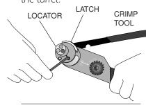
Select the proper locator position for your contact by rotating the locator until the proper color is aligned with the index mark. Push locator back down until it snaps into position.
