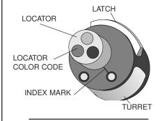
4. Adjust dial for proper wire gauge. To change the dial setting, remove the lock pin and lift center of dial. Turn to the desired wire gauge. Replace lock pin on dial.
