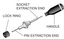
3. On the mating face of the connector, insert the tool over the pin contact or into the socket contact until the tool bottoms. Apply a slow continuous pressure to push the contact out the rear of the connector. When the shoulder of the tool "thunks" against the insulator, the contact is extracted.
