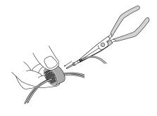
4. Place the connector into an assembly fixture (fixtures are available for production use, call us.) If you are not using a fixture, be sure to allow clearance on the mating face of the connector for the guide pins to come through the connector during insertion.
