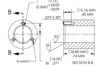
SECURE WITH APPROPRIATE LENGTH M4X0.7 FASTENERS
