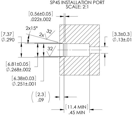
RECOMMENDED RETAINING RING TRUARC N5000-25 OR EQUAL REPLACE O-RING IF REMOVED FROM PORT
