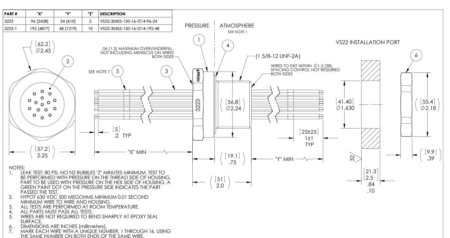
8. COSMETIC SURFACE VOIDS NOT ON O-RING SEALING SURFACES ARE ACCEPTABLE BASED ON THE SEAL'S DIAMETER:
