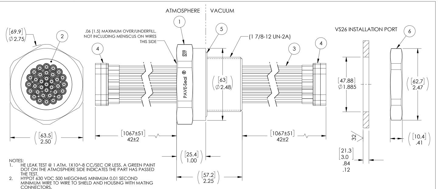
3. CONTINUITY TEST WITH MATING CONNECTORS: SHIELDING < 1.0 OHM END TO END
