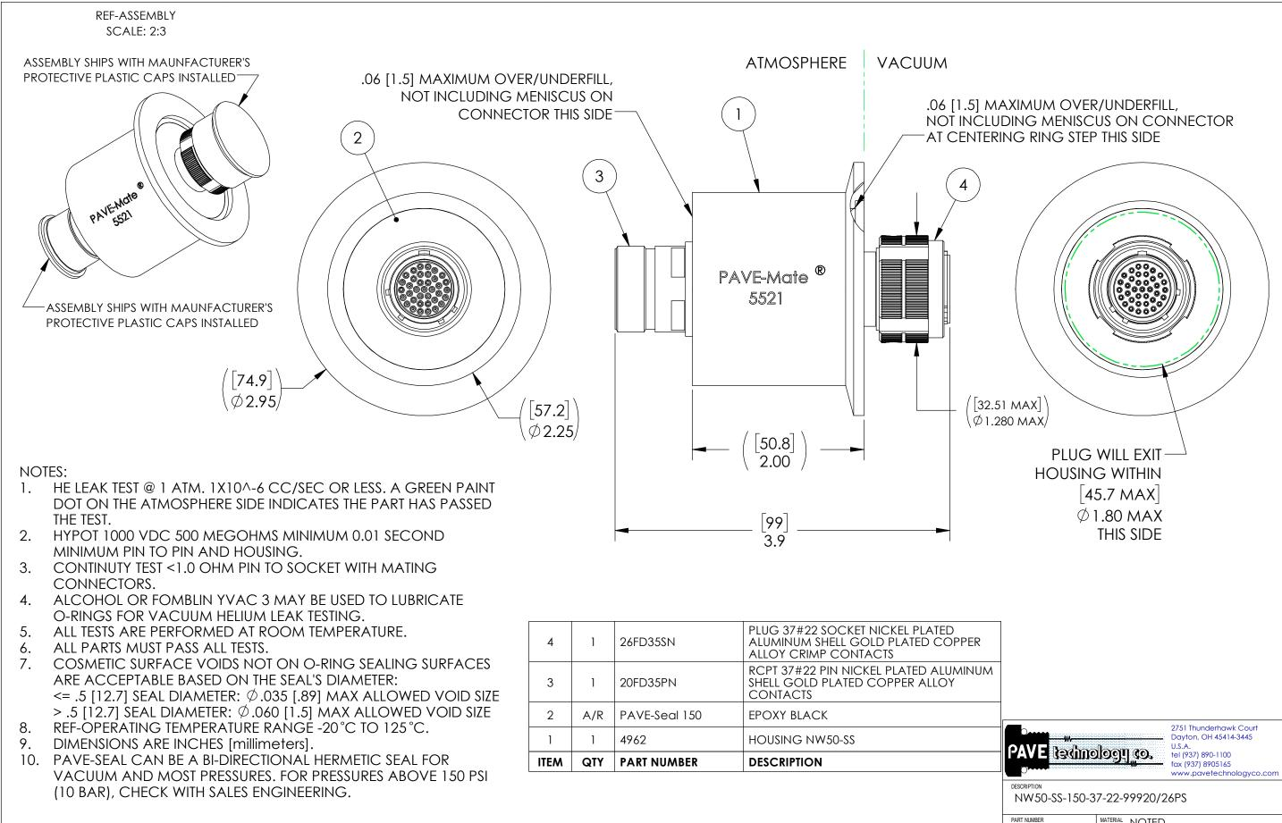
ALL DIMENSIONS AND TOLERANCES APPLY TO FINISHED PART IN INCHES. ALLOWABLE TOLERANCES UNLESS SPECIFIED OTHERWISE: NONE ±0.5 X.X DECIMAL ±0.1 X.XX DECIMAL ±0.02 X.XXX DECIMAL ±0.005 ANGLES ±1 DEGREE SURFACE FINISH 128 microinch RMS
